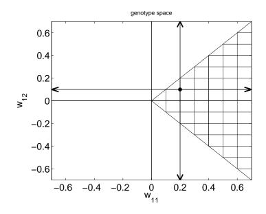
Figure 3: A particular discretization of the  $(w_{11}, w_{12})$  where  $w_{1i} \in \{-.7+0.1m | m = 0, ..., 14\}$ . Since the other points have fitness zero, we keep track of the states within the triangular region in the *G* matrix only. However transition probabilities are evaluated on the basis that a state can move to anywhere in the square moving in a horizontal or vertical direction after a mutation.
