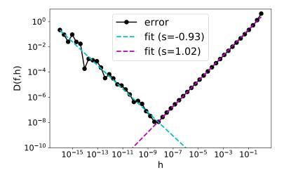
To avoid the disastrous (unreliable or error-prone) behavior, we must take  $h \gg 10^{-8}$ . The minimum error possible is around  $10^{-8}$  also - it cannot be made arbitrarily small. However, when h is above this threshold, the error scales like Ch (which is good to know).
