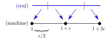
Moreover (guaranteed by implementation on processors),  $\epsilon_m/2$  represents a bound on the relative error in basic arithmetic on the computer. The value  $\mathbf{u}_m = \epsilon_m/2$  is called the rounding unit.
