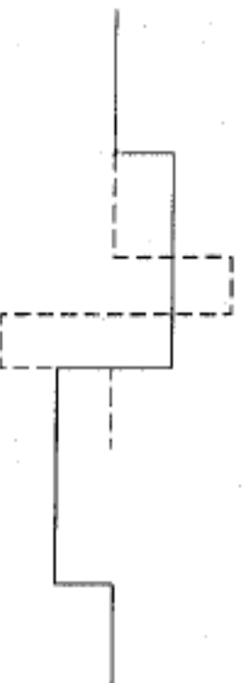
FIGURE 5. Two Haar wavelets; the support of the "narrower" wavelet is completely contained in an interval where the "wider" wavelet is constant.
