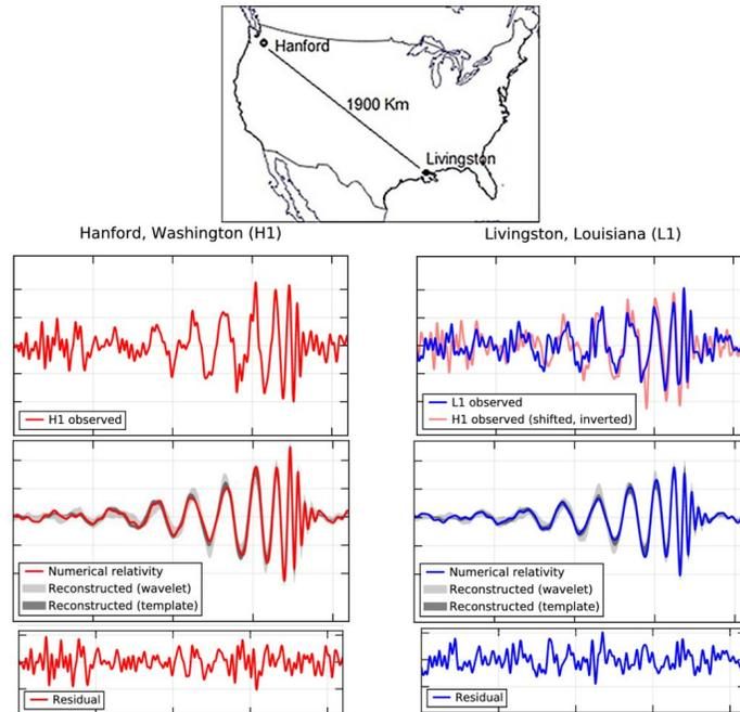
Figure 5. The graphs show the results of GW150914 recorded at both LIGO sites. The top graphs are the recorded events, the middle graphs are the expected graph for black hole merger, and the bottom graph is the random noise caused by thermal fluctuations (Cervantes-Cotes, 2016).
