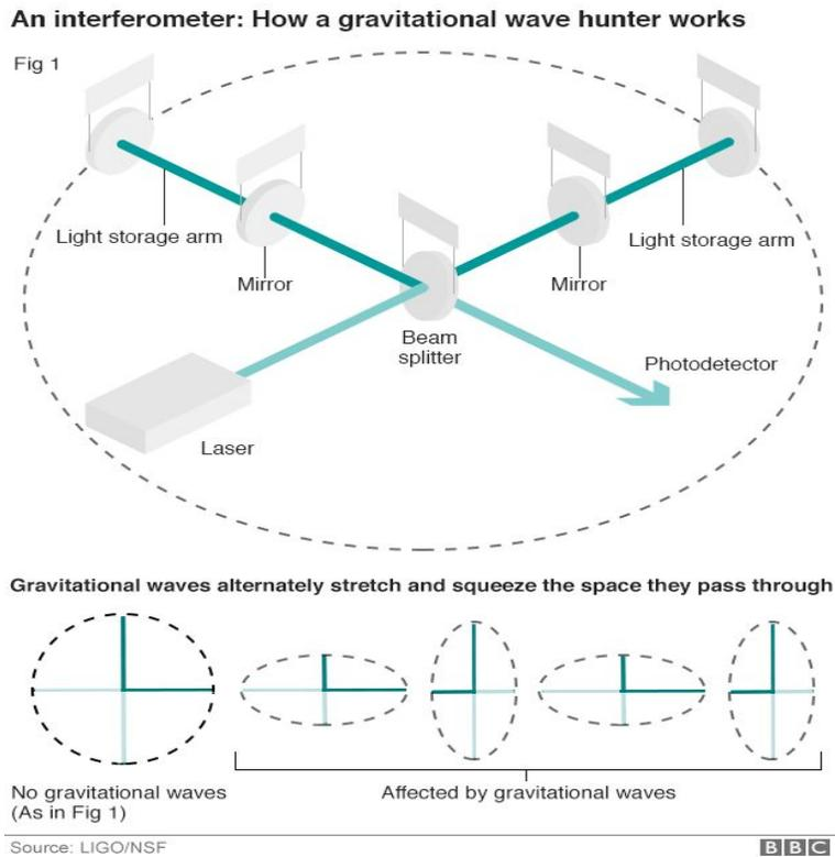
Figure 4. The top diagram shows the setup for Advanced LIGO. The diagram is similar to that for a Michelson interferometer except LIGO has an extra mirror in between the beam splitter and the end mirror for the arm (Amos, 2016).
