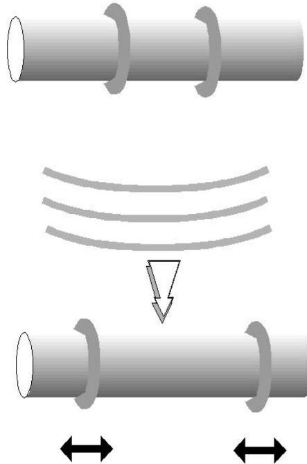
Figure 3. The sticky bead argument. The top picture shows a cylinder with two rings around it and the bottom picture shows a gravitational wave passing through the system, resulting in movement of the rings and thus causing friction. (Cervantes-Cota, 2016).
