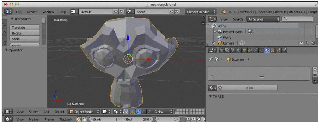
This will create a new material and assign it to our monkey geometry. If you scroll down in the material tab after the material has been created, you can set some Three.js-specific properties, such as the material type to be used and the type of blending you expect. This is shown in the following screenshot:
