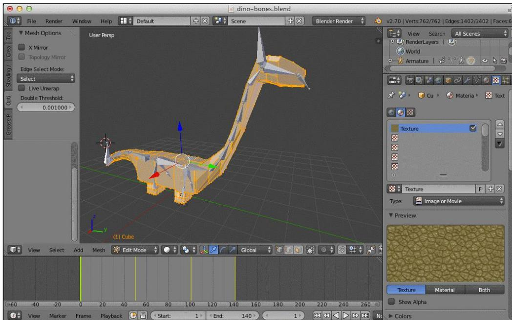
In this screenshot, you can see the shape of the dinosaur and also the skeleton it is made of. For this example, we've connected the model to the bones you can see. The result is that whenever we move the bones (in the pose mode in Blender), the model deforms as well. We've used this to create a number of poses for this dinosaur. One of the poses is shown in the following screenshot:
