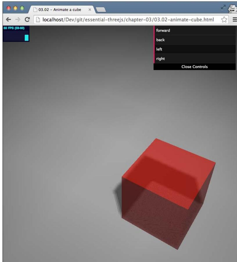
Using the controls at the top-right corner, you can move the cube around. What you'll see is that the cube rotates around its edges, not around its center. In this section, we'll show you how to create that effect. Let's first look at the default rotation, which is along an object's central axis, and the translation behavior of Three.js.
