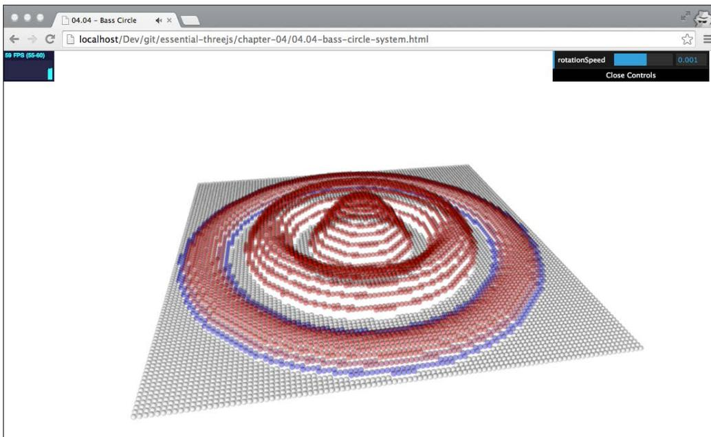
In this screenshot, we've got a particle system that shows the volume of the low, mid, and high ranges. In the middle of the screenshot, you can see the volume of the low range. The middle ring shows the volume of the mid range, and the outer ring shows the high notes.
