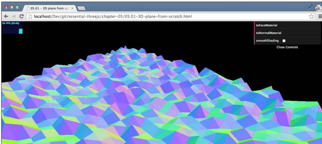
In this example, you can also enable `smoothShading`. With `smoothShading`, you don't see the individual faces, but Three.js combines them to create a smooth geometry. You can easily enable this by setting the `shading` property of the material to `THREE.SmoothShading`. The result looks like the following screenshot:
