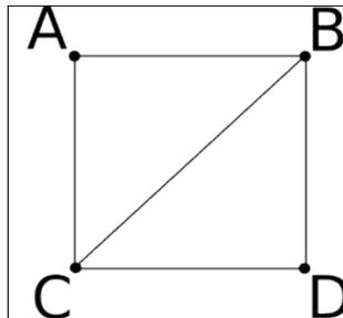
As you can see in the figure, we are going to create squares by combining two faces. So we need to create a face using the **A**, **B**, and **C** vertices, and another face using the **B**, **C**, and **D** faces. We do this in the following code fragment:
