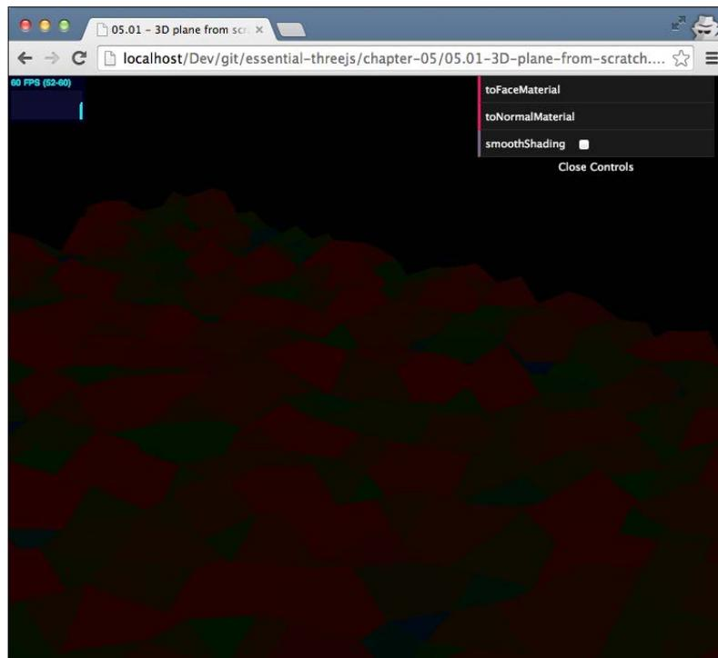
The shapes seem to be there, but the lighting and shading is completely off. The reason for this is that Three.js is still missing one piece of information. What we need to specify is the face normal vector. This is the vector that is perpendicular to the face. This is used by Three.js to determine how lighting applies to this specific face. We could calculate this by hand, but luckily Three.js provides an easier approach for this. Have a look at the following line of code:
