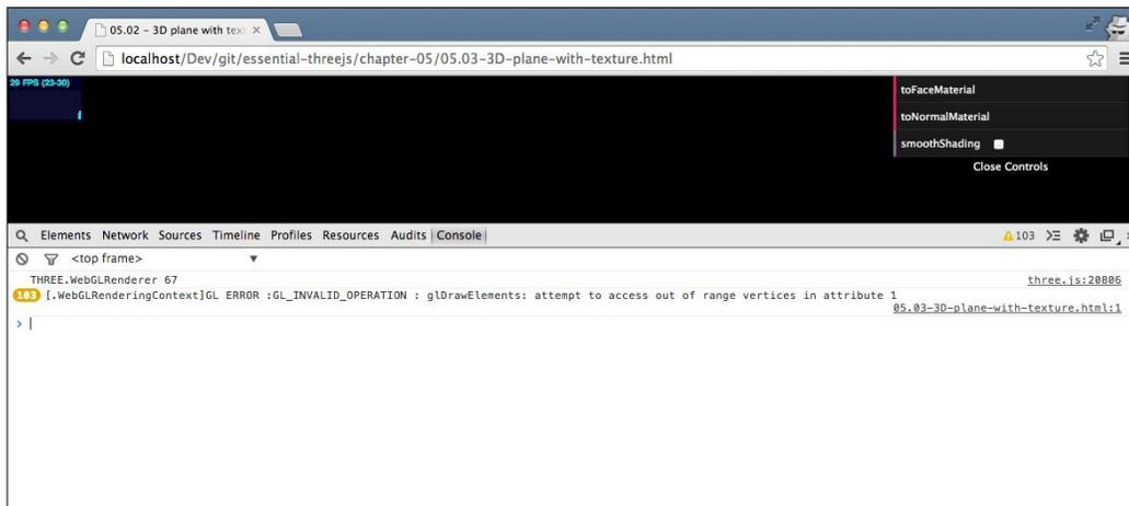
The reason, which isn't actually clear from this error message, is that we're missing one more piece of configuration in the geometry we've created: the UV map.
