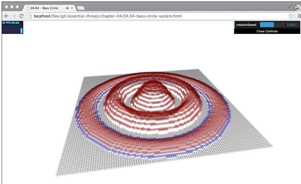
The visualization you can see in the previous screenshot shows the low, mid, and high tones of the audio that is being played in the form of concentric circles. The low tones are shown in the center of the visualization, the second circle shows the mid tones, and the outermost circle shows the amplitude of the high tones. To create this visualization, we have to perform the following steps:
