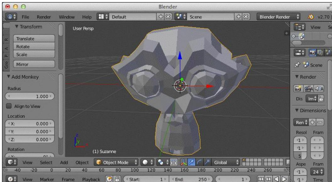
Now that we've got a model in Blender, we can use the plugin we installed at the beginning of this chapter to export this model to Three.js. To do this, go to the **Export** | **Three.js** option from the top menu, as shown in the following screenshot:
