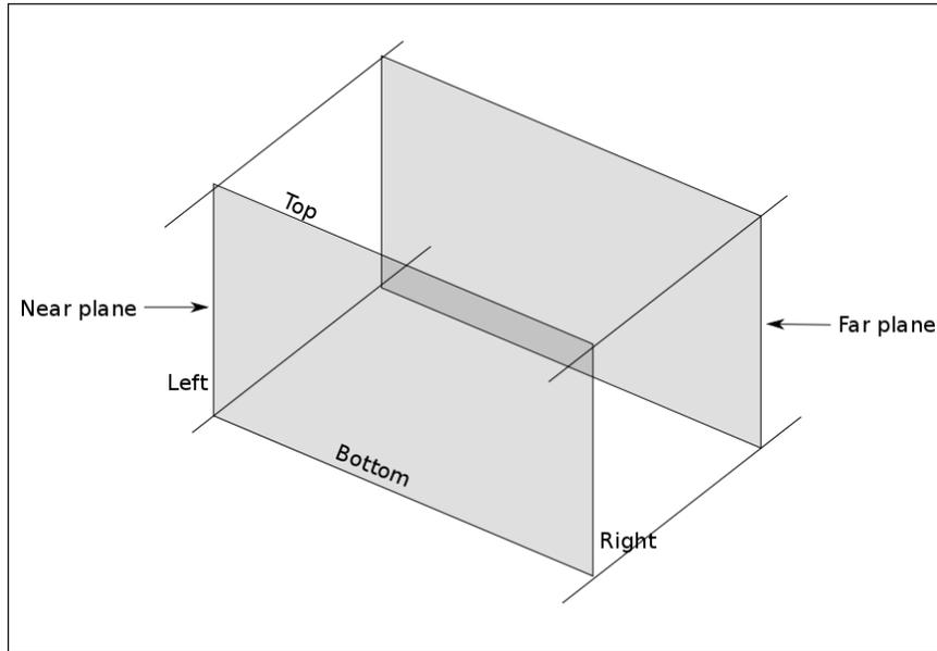
Here, you can see the cuboid area that we defined, and this is rendered when the orthographic camera is used. Now, let's create a new scene and add a 2D plane (`THREE.PlaneGeometry`) with a starry background as the texture. This is described in the following code:
