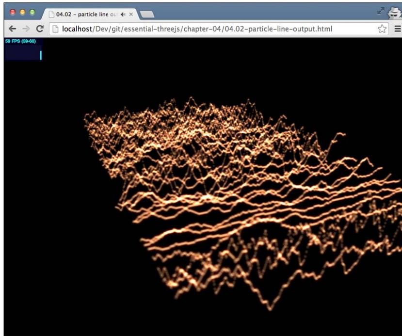
To accomplish this sound visualization, we need to perform pretty much the same steps as we saw in the previous example. We need to configure our audio. Next, we need to access a `NodeAnalyser` interface to get the waveform; based on this information, in this example, we're going to create a new particle system.
