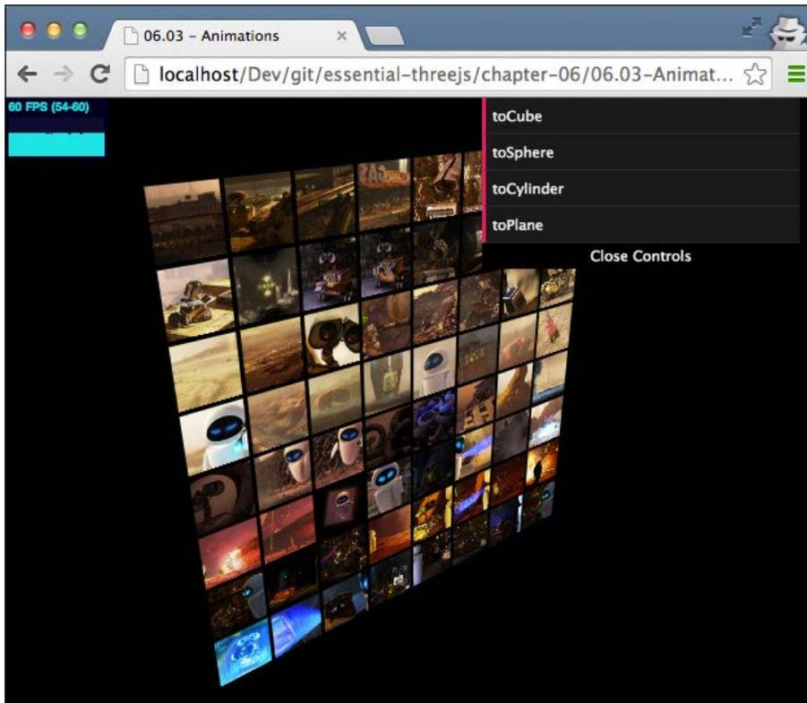
If you run this example, you'll see a rotating 3D object built up from a number of images. Using the menu on the top right-hand side of the window, you can change the shape of the 3D object, and the various components will automatically move to their correct new position and rotation. Let's start with the beginning and look at the HTML element that we use to show the image.
